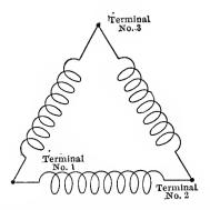
FIG. 67. Diagram of " $\Delta$ " or mesh connection of the three armature windings of a three-phase armature.
